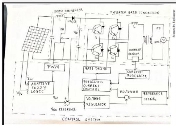
**Fig1:-PV grid with multilevel inverter and neuro system.**
